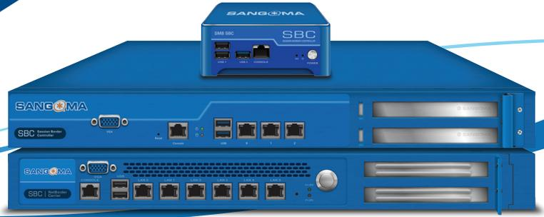
Sangoma's Session Border Controller (SBC) product line is designed to provide SMBs, enterprises and service providers with unbeatable VoIP protection. SBCs connect businesses to ITSPs, remote workers, and SIP endpoints securing all VoIP traffic that passes through the environment.
